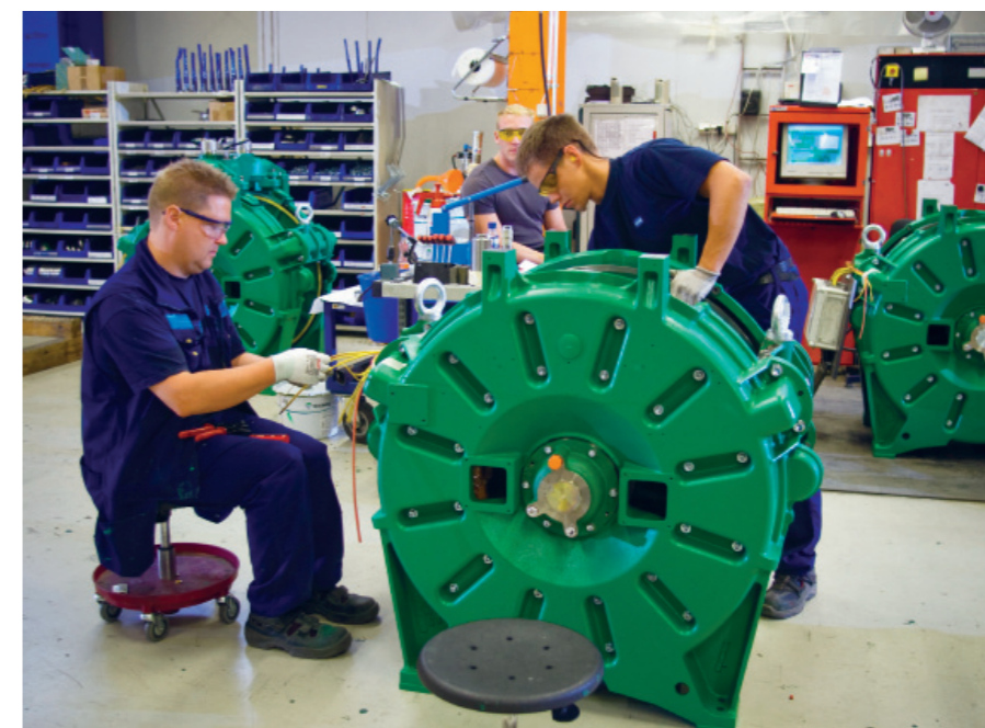
The KONE EcoDisc® hoisting machine contains no oil.
