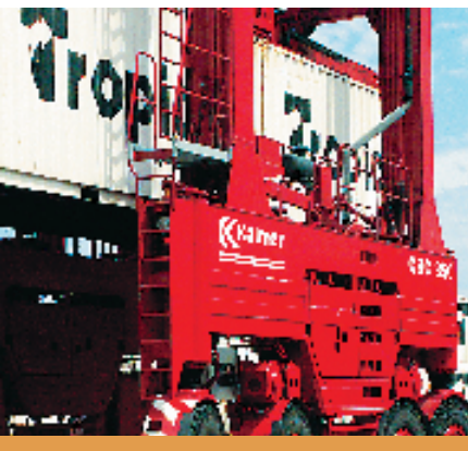
The 15 meter high Kalmar straddle carrier can stack containers in 4 stories.
