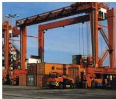
RTG's, RMG's Finland and Shanghai
