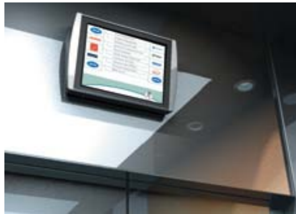
The OPC interface is used to deliver information on in-car flat screens. This helps to guide visitors and staff using the elevators.
