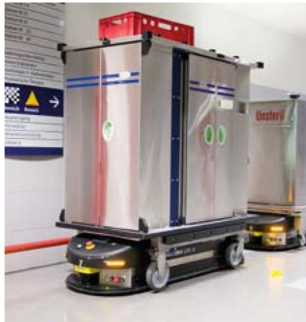
AGVs are automatic guided vehicles that navigate unmanned through the hospital. When needed, the AGV calls the elevator via WLAN and OPC interface and changes the elevator to 'freight service mode'. The elevator serves the current passengers and goes to the floor where the AGV is waiting. The AGV then enters and requests a floor. Upon arrival, the AGV drives out and the elevator returns to normal mode.
