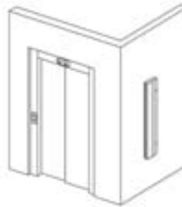
MAP mounted on side wall: Aluminium (A) or Asturias Satin (F) stainless steel
