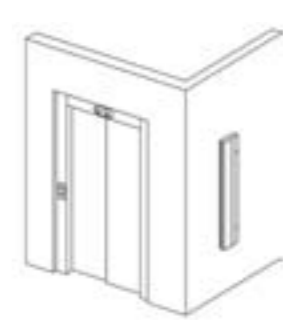
MAP mounted on side wall: Aluminium (A) or Asturias Satin (F) stainless steel
