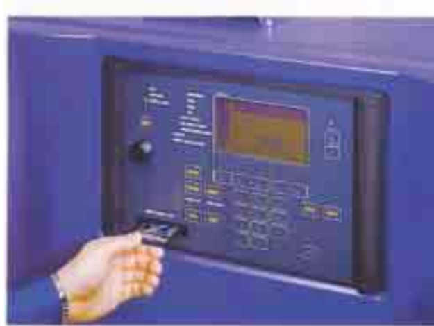
Fig.10 TMS9900 GA Operator Interface panel
